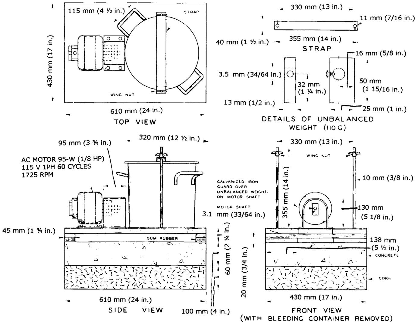
FIG. 2 Detail of Vibrating Platform Apparatus
